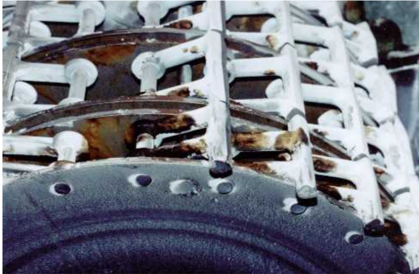
Figure 1 Scorched hammers in a hammermill.
