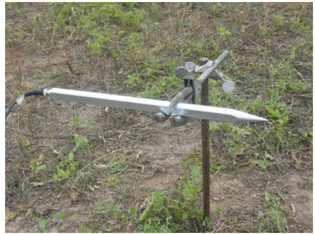
Figure 3. Blast wave transducer
