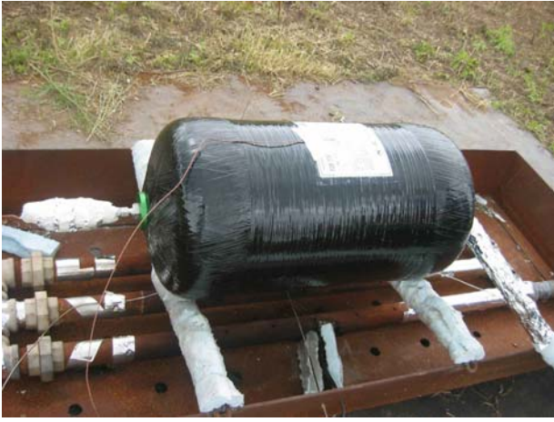
Figure 1. Hydrogen Tank Prior to Test
