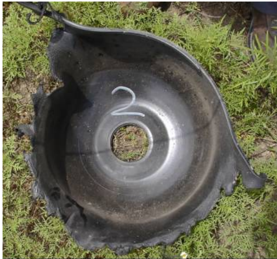
Figure 7 Cylinder dome end cap projectile.
